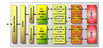
Figure 1: Block diagram of a Dual-Core Intel Itanium2 (Montvale) processor.
