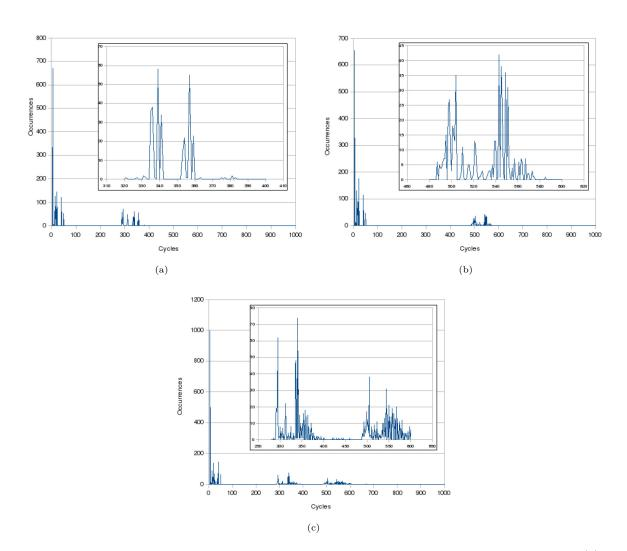
Figure 3: Latency of memory accesses when the data is allocated in memory local to the core (a), in memory on the other cell (b) or in the interleaving zone (c). The y-axis shows the number of occurrences of every access. The x-axis shows the latency in cycles per memory access. Regions of interest have been zoomed in.
