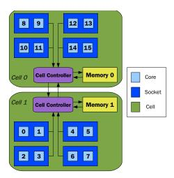
Figure 2: Block diagram of a rx7640 node.
