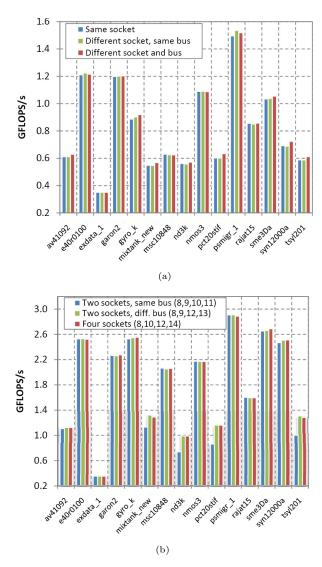
Figure 5: Influence of the thread allocation on a rx7640 node: using two (a) and four threads (b).
