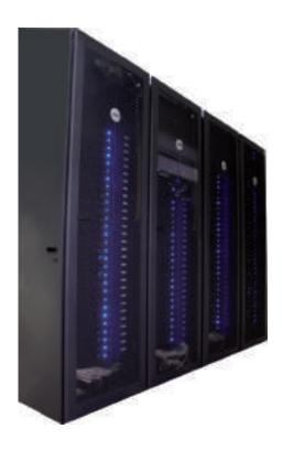
CESGA offers server architectures designed to solve a high number of problems of minimal computational complexity in a short period of time. The HTC servers, High Throughput Computing, incorporate a large quantity of scalar processors with rapid access to a local memory of limited size. These servers have an internal network of interconnection with medium-high latency.
