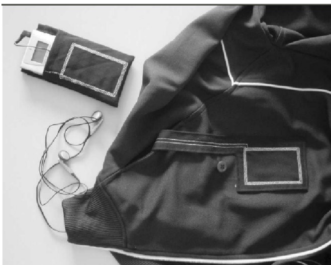
Fig. 4. Wireless connection between MP3-player and the on-shirt textile connection to the earphones using sewed textile coils.
