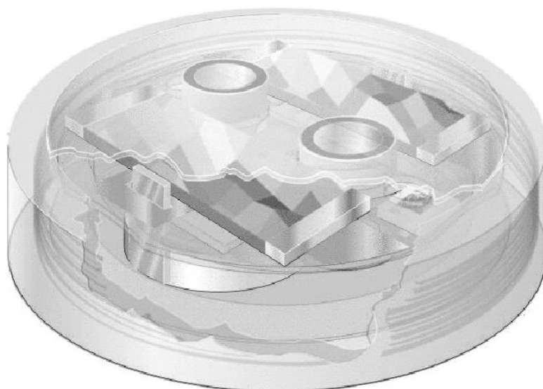
Fig. 6. Design of an autonomous 'sensor button', diameter 15mm, height 5mm [35].
